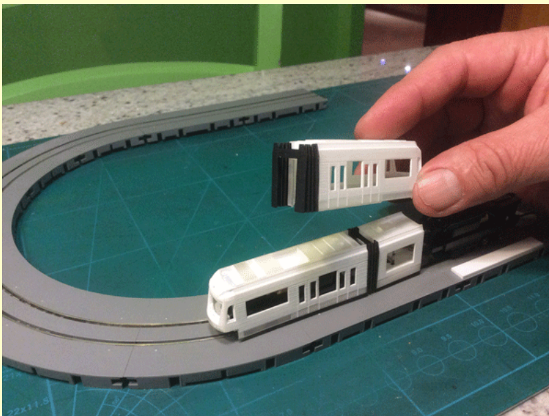
The first or Beta unit prior to painting showing the articulation bellows made from folded black paper.
