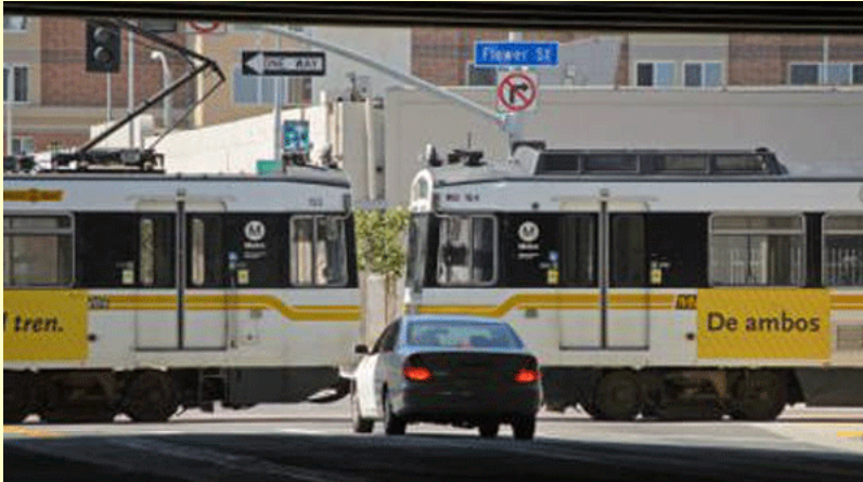
Two 1995-built P2020 NipponSharyo LRVs at a Grade Crossing in downtown Los Angeles!
