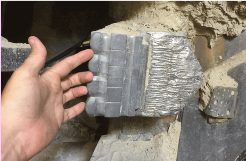
Worn out part - close view of one worn cutter head element!
