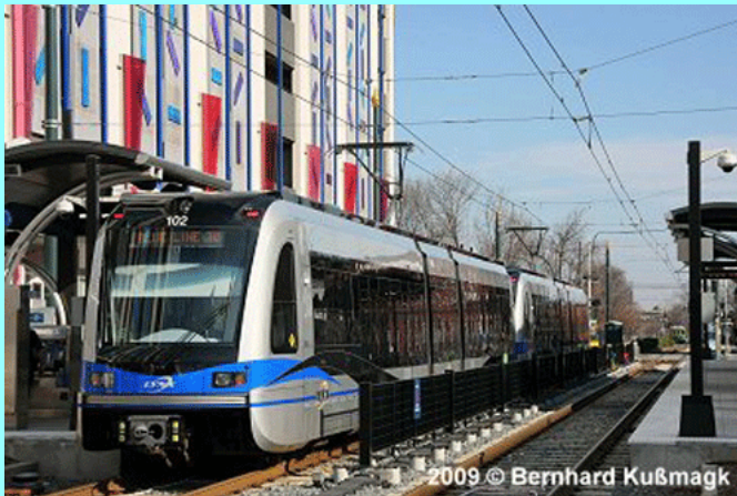
One of CATS original 16 Siemens S70 Partial Low Floor Light Rail Vehicles!
